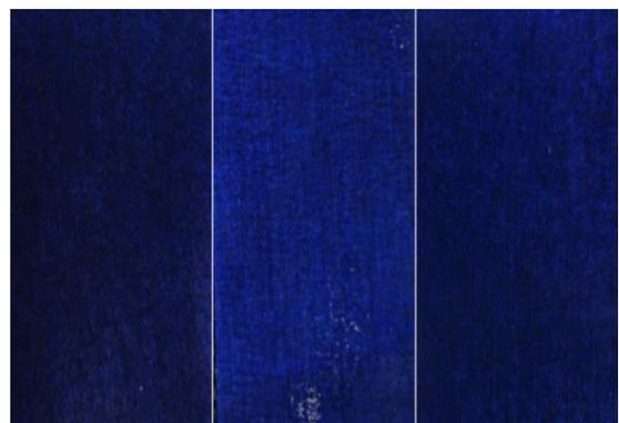
**Figure 3: Photographs of the coating film during inking (left: Emulsion B, middle: Emulsion B / Rosin mixture, right: PE-2189)**
