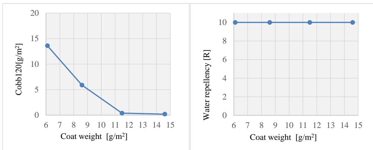
**Fig. 4. Relationship between coat weight and water resistance of papers coated with T-EF104 (drying condition: 100°C-30 s)**
