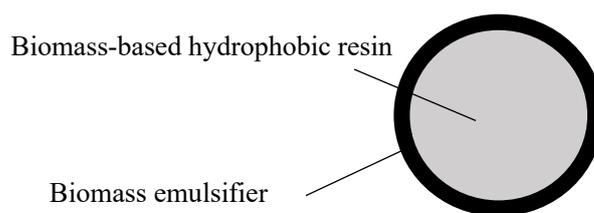
**Figure 1. Image of particle structure of T-EF102 and T-EF103 emulsions**
