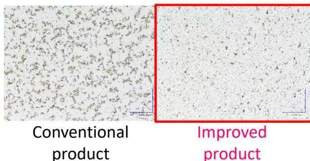
**Figure 8.** A comparison of images showing the degree of coagulation when conventional and improved product are diluted
